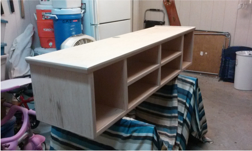
ALAN WENDEL This is an open shelf Alan made for his sister and brother-in-law. It is made out of maple plywood (leftovers from the workbench the club members made). It is finished in espresso. The backs of the shelves have extra cut outs to allow for all of the cords to be hidden.
