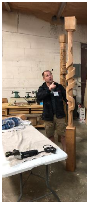
You can see by the horizontal lines that he cuts each with that cutter laying on table. Then chips out all the wood. Then does it all over again till he has the profile of the snake standing out from the wood pole.
