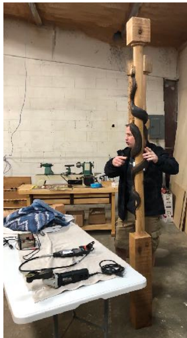
You can see by the horizontal lines that he cuts each with that cutter laying on table. Then chips out all the wood. Then does it all over again till he has the profile of the snake standing out from the wood pole.
